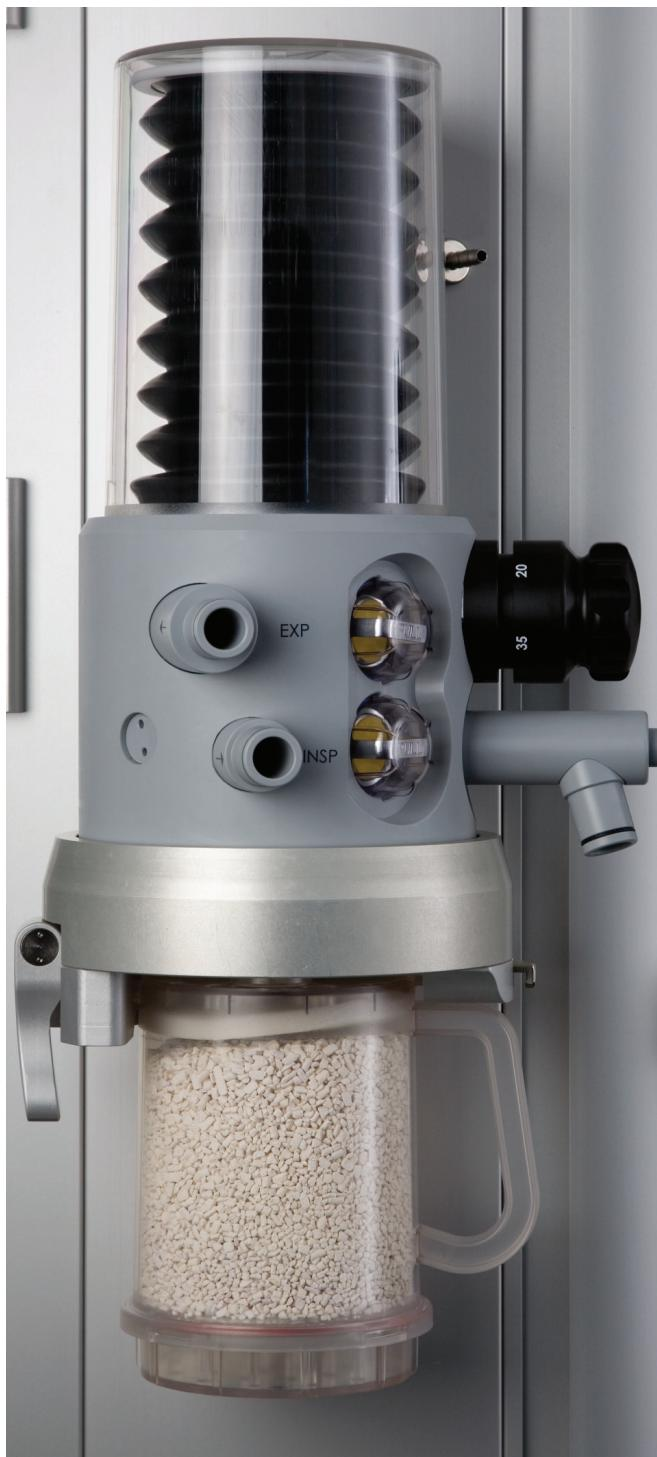
Forget about time-consuming, multiple tubing connections between the anaesthesia machine, patient system and patient. Our integrated breathing system (IBS) integrates an ascending bag-in-bottle, patient circuit and CO<sub>2</sub> absorber in one compact unit.
